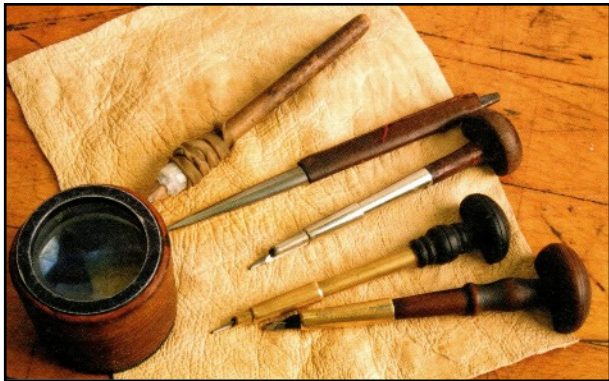
Using the sort of tools shown on the left, an engraver cut an intaglio image into a steel master die.
