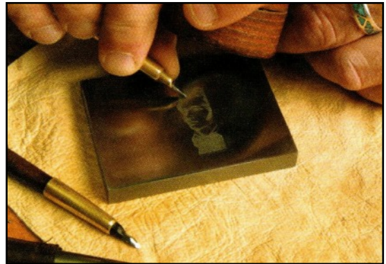
Using the sort of tools shown on the left, an engraver cut an intaglio image into a steel master die.
